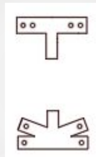
Figure 1: Mid-Span Top and Bottom Chord Gusset Plate Connections
